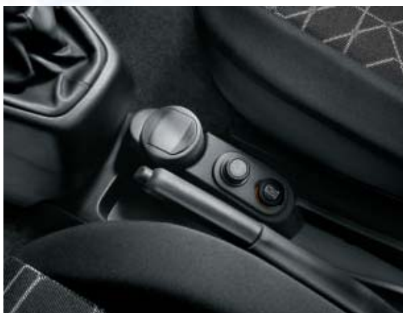
Central cabinet unit with ash-tray/glass holder, cigarette lighter and 12V socket.
