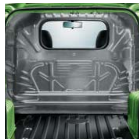
Glazed partition between the cab and the loading compartment.
